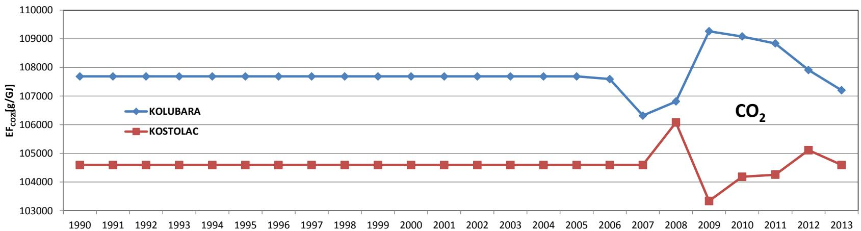
Average value of CO<sub>2</sub> emission factors for lignite from Kolubara basin, according data presented in this report, is 107685 g<sub>CO<sub>2</sub></sub>/GJ, while net calorific value is 7975 kJ/kg.
